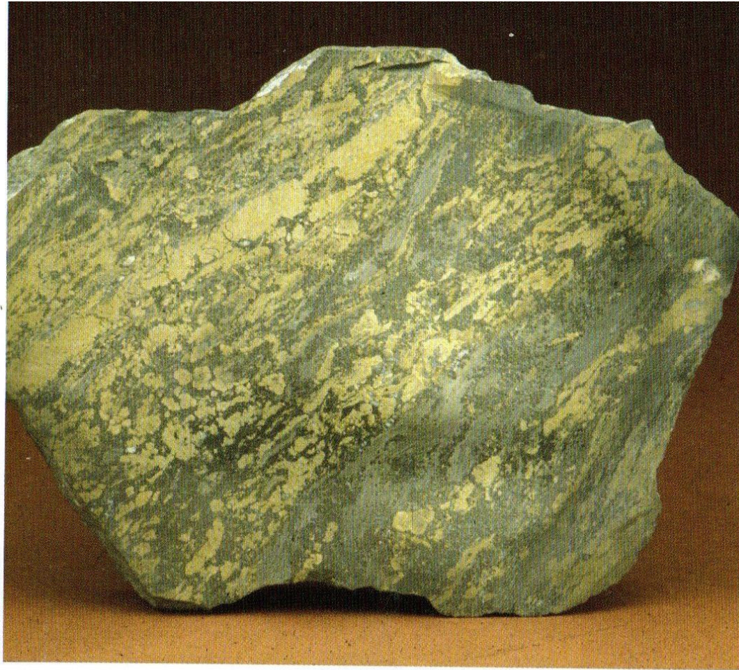
Figure 4.14 Pyrite mineralization in dark, metalliferous sediment — from the sulphide deposit at Parys Mountain, Anglesey. Field of view 18 cm across.
